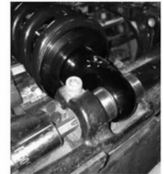
Wide Bearing Spacers with O-Rings installed as shown and installed at rear shock mount (swingarm).
