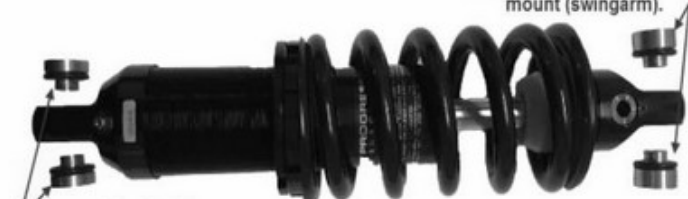
Narrow Bearing Spacers with O-Rings installed as shown and installed at front shock mount (frame).
